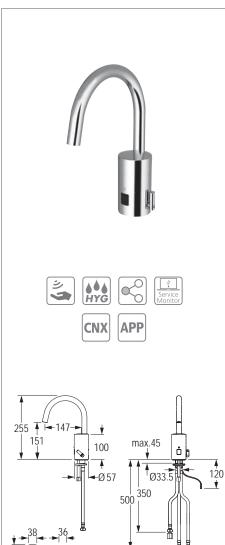
loopino lavatory faucet G30, with IR sensor, with temperature-mixing, pressureless (for open water heater), chromed
