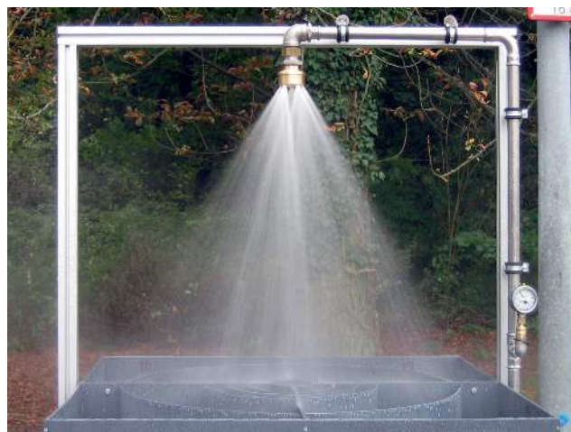
Normenconforme waterverdeling van de NovaLab-nooddouchekop
